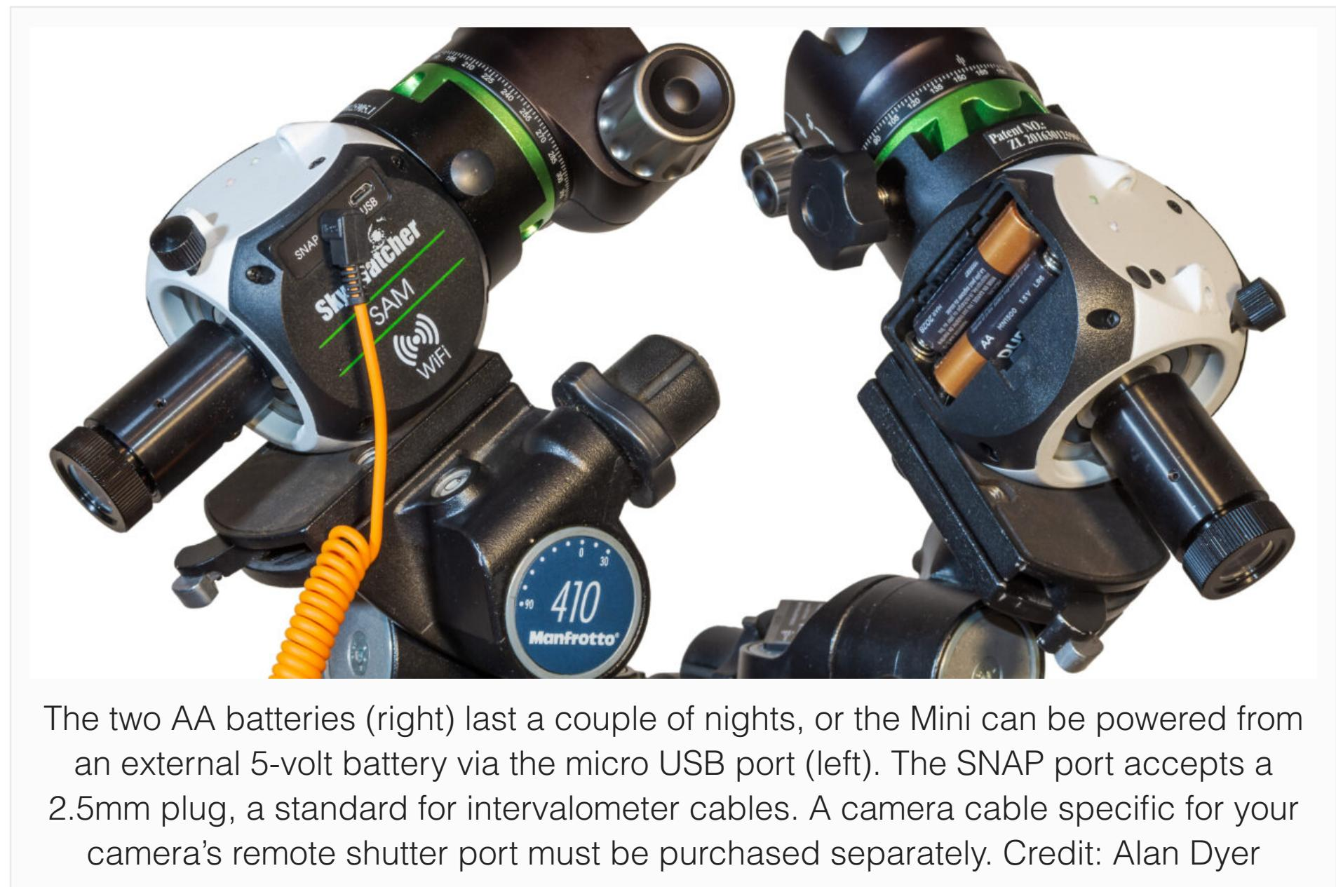
The two AA batteries (right) last a couple of nights, or the Mini can be powered from an external 5-volt battery via the micro USB port (left). The SNAP port accepts a 2.5mm plug, a standard for intervalometer cables. A camera cable specific for your camera's remote shutter port must be purchased separately. Credit: Alan Dyer
