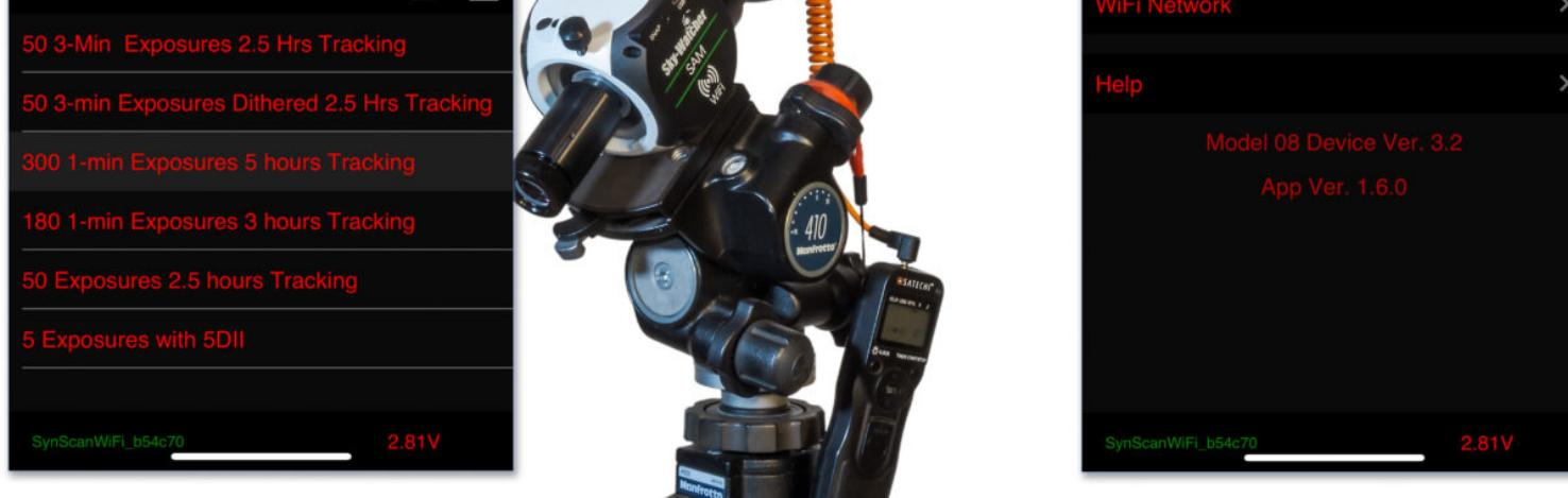
The SA Console app's various modes (Astrophotography is at left) allows setting exposure time, interval and frame count, plus saving combinations as user presets. The Settings page (right) has the option for Auto-Run Task, avoiding app use each night. Credit: Alan Dyer
