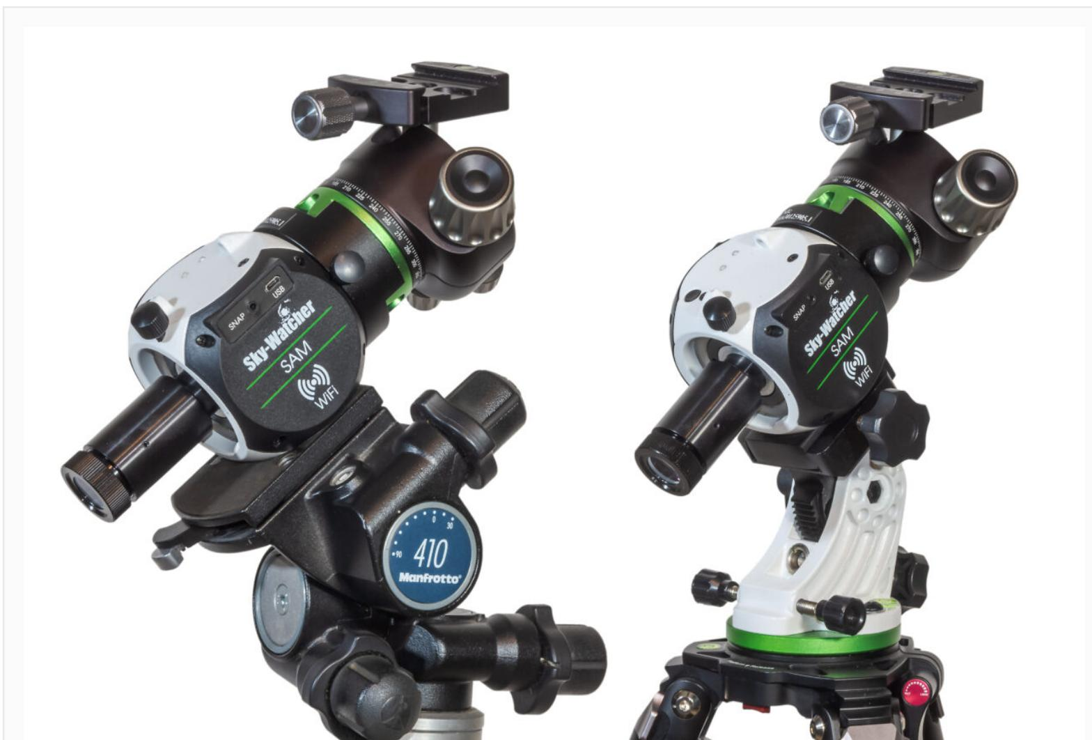
The basic Star Adventurer Mini is mounted on a tripod head (left) but using a three-axis head is a good option for ease of precise polar alignment. The Pro Pack comes with the solid EQ Base (right), which has its own fine adjustments for polar alignment. Credit: Alan Dyer
