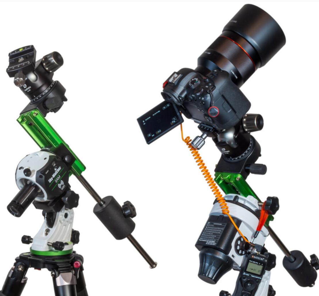
A Mini (left) accepts the same accessories as the larger Star Adventurer 2i (right). The Mini's Pro Pack includes the Latitude EQ Base and Declination Bracket, but not the Counterweight kit shown. For most uses the Declination Bracket will not be needed. Credit: Alan Dyer
