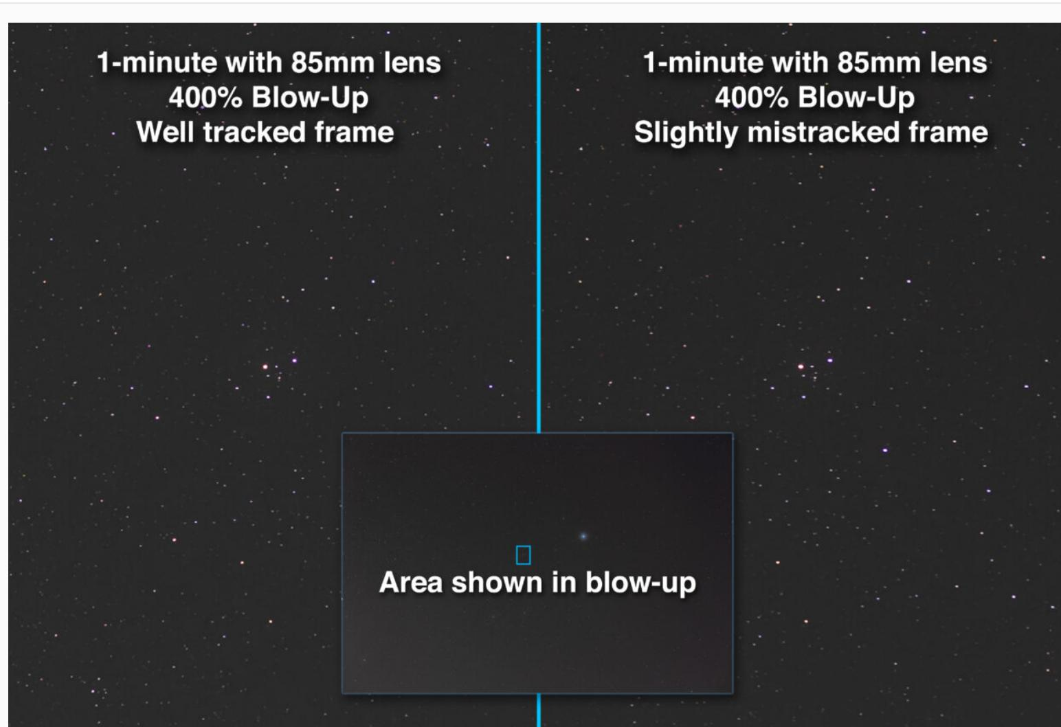
Extreme blow-ups of two frames with an 85mm lens showing the tracking accuracy extremes out of 100 frames.. Credit: Alan Dyer
