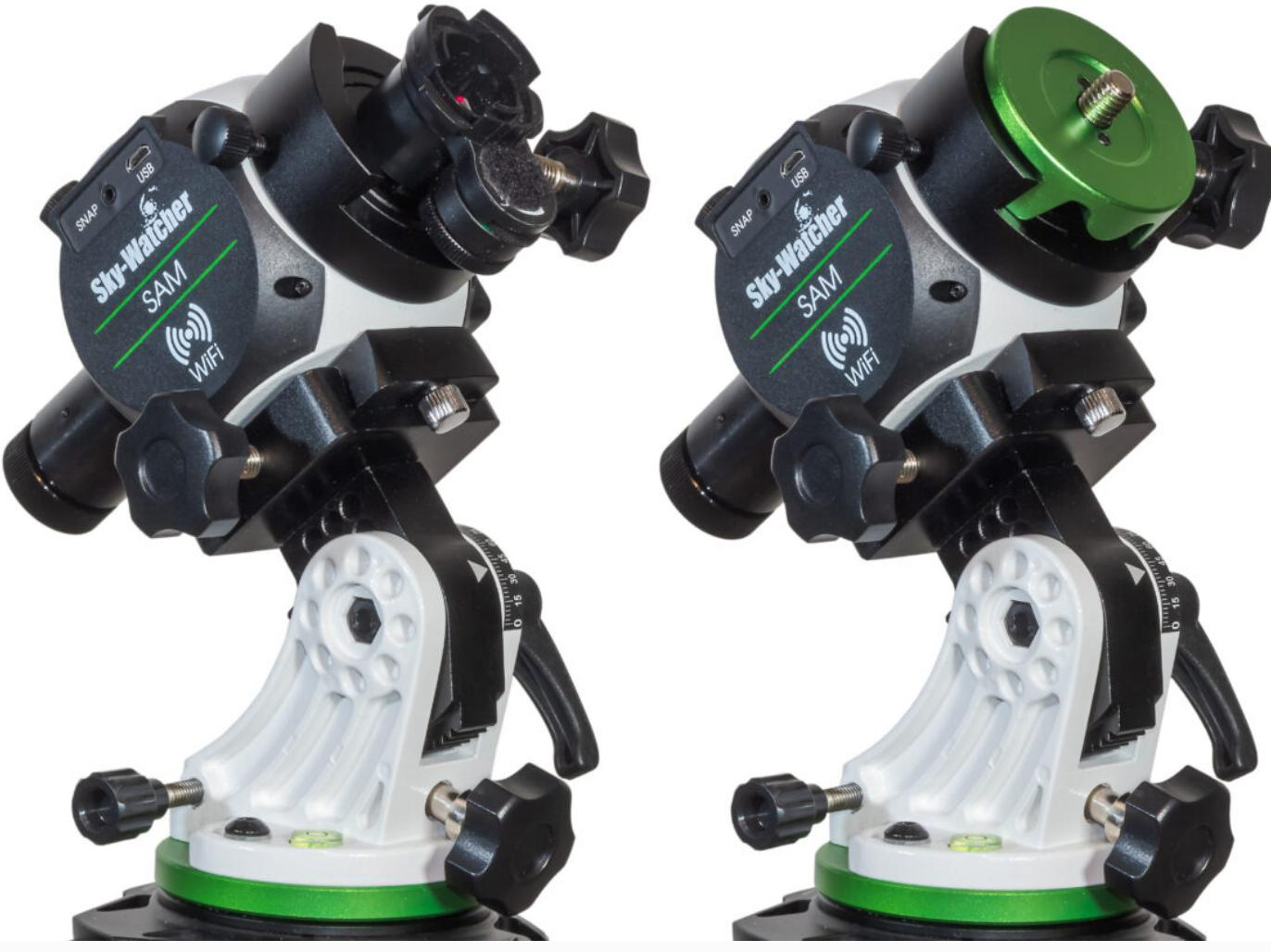
Seeing the polar alignment reticle requires the included illuminator (left), which has to be removed before the ball-head adapter plate goes on (right), blocking the polar scope's view of the sky. A ball head, as shown in other photos, is user-supplied. Credit: Alan Dyer
