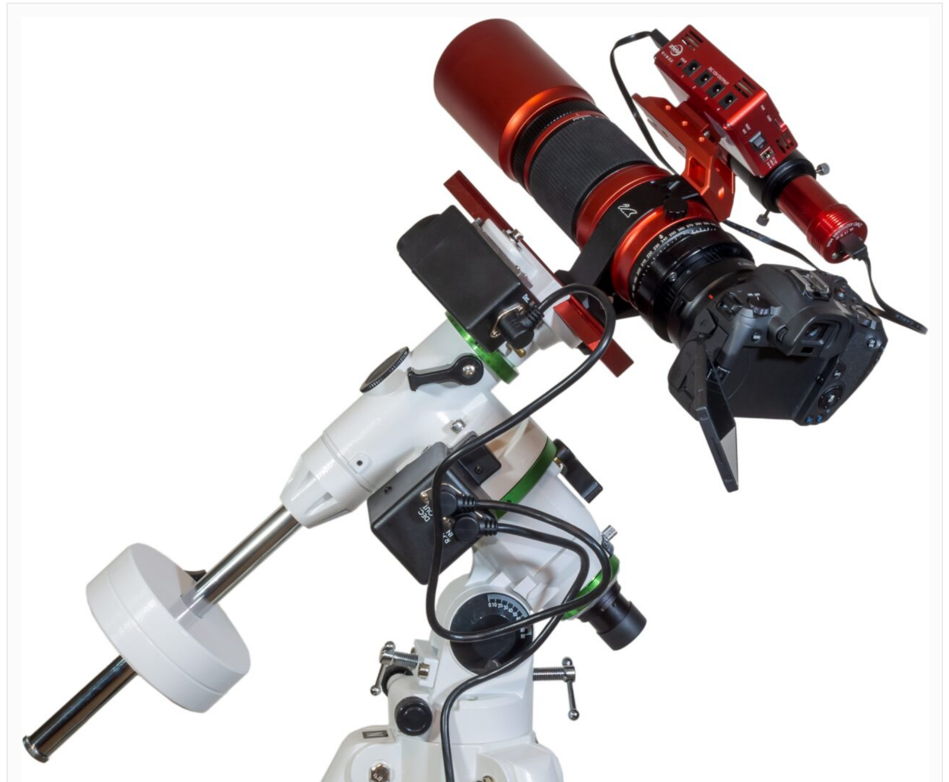
The EQM-35 is ideal for small astrographs such as the William Optics RedCat 51mm, shown here with a ZWO ASlair and ZWO guidescope and camera for autoguiding.
