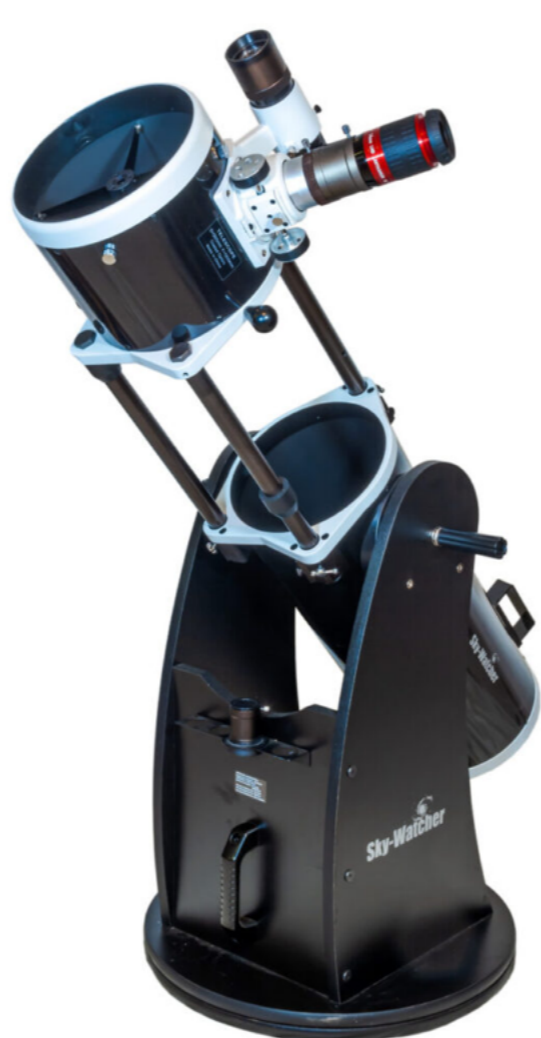
The Sky-Watcher Flextube 200P with a 2-inch eyepiece and the magnetic counterweight described in the text. Current telescopes have white mounts. Credit Alan Dyer
