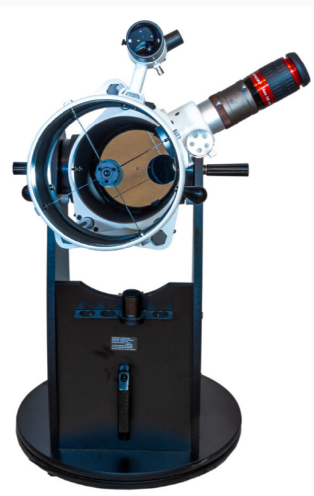
The four-vane spider is solid and the primary mirror is center-marked for ease of collimation. A knob near the eyepiece aids in moving the telescope. Credit: Alan Dyer
