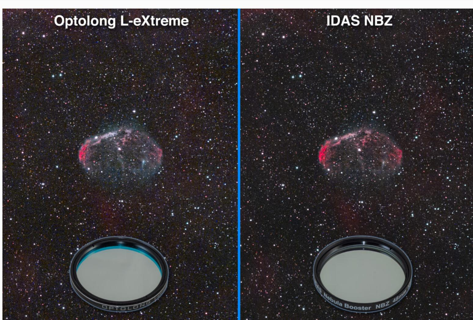
The L-eXtreme revealed more O III emission than the NBZ. Either filter could be used just to collect images primarily for the O III content, with the Ha content coming from images shot with one of the wider bandwidth filters. Images shot without a filter can add the natural star colors. Credit: Alan Dyer
