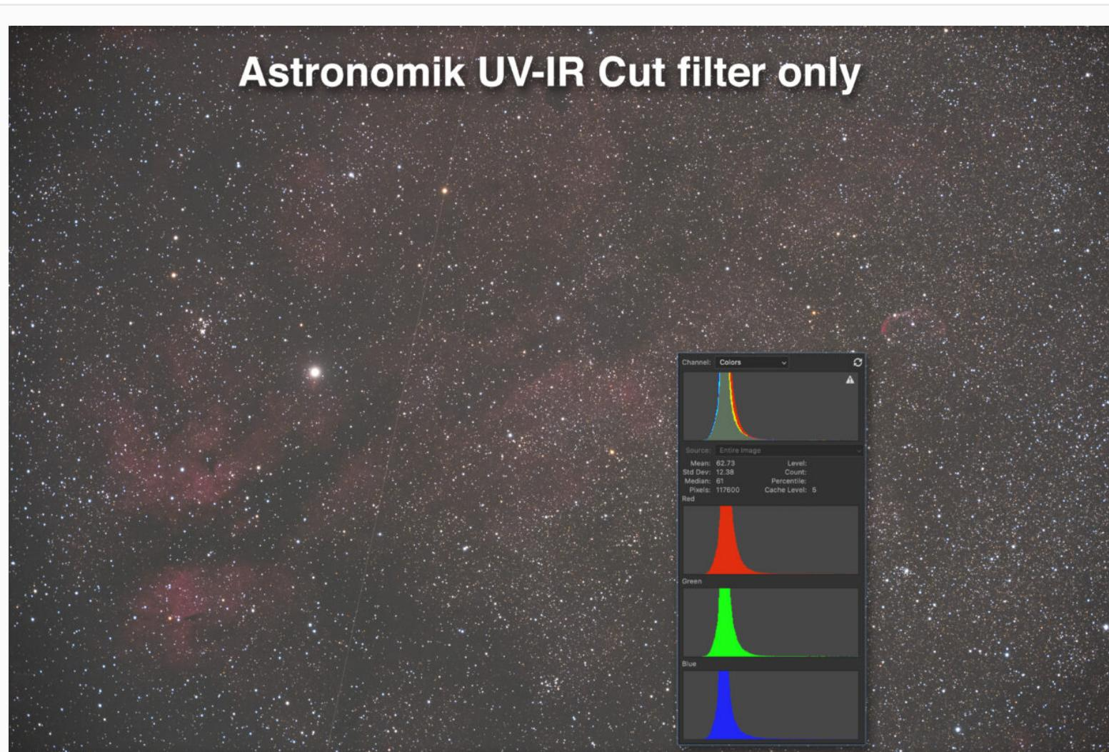
This shows a single “white light” image taken in a dark sky with no light pollution filter, for comparison. It records nebulosity, but not to the extent possible with a narrowband filter. The inset histogram graphs the exposure in this “out-of-camera” raw image. Credit: Alan Dyer
