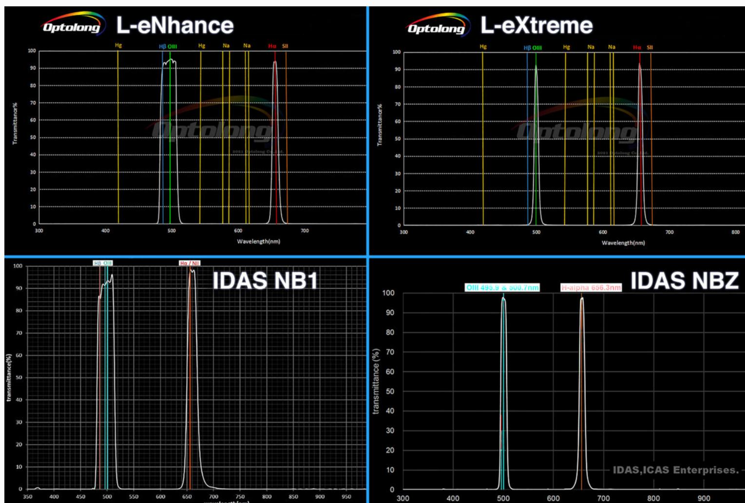
The transmission charts supplied by Optolong and IDAS show the filters' bandwidths, with the L-eXtreme and NBZ having narrower passbands than the other two filters. All four are more restrictive in bandwidth than typical Ultra High Contrast (UHC) filters. Credit: Adapted by Alan Dyer from originals by Optolong and IDAS
